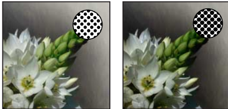
Proof (no dot gain), and printed image (with dot gain)
